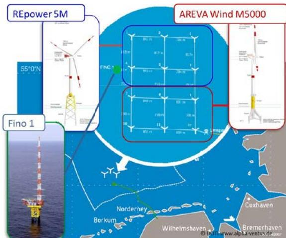
Figure 1: Location and layout of alpha ventus; also shown are the turbine types and the FINO 1 research platform (© artwork: DOTI; © picture: DEWI)
