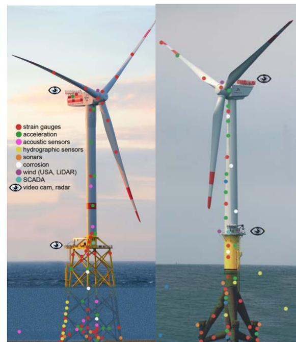
Figure 2: Sketch of Repower 5M (AV4; left) and AREVA Wind M5000 (AV7; right) offshore wind turbines in the alpha ventus test site. Markers indicate locations and type of instrumentation used for the RAVE measurements. (© pictures: DOTI; Editing: Fraunhofer IWES)
